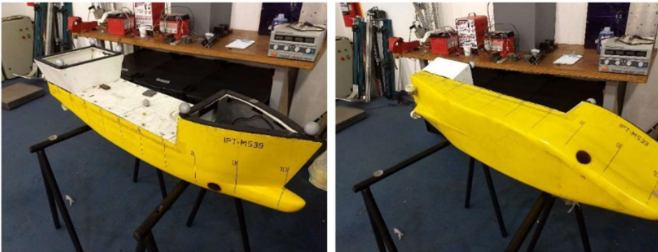
Figure 5.2: PSV scale model used during the experiments (Ianagui 2019).
