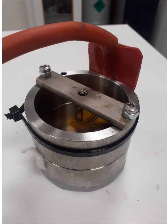
Figure 3.12: Experimental setup for measurement of thermal conductivity of solid PCM samples
