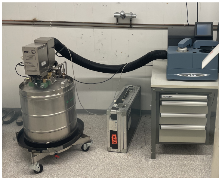
Figure 3.8: TA Instruments Q2000 differential scanning calorimetry equipped with liquid nitrogen cooling used for PCM characterisation
