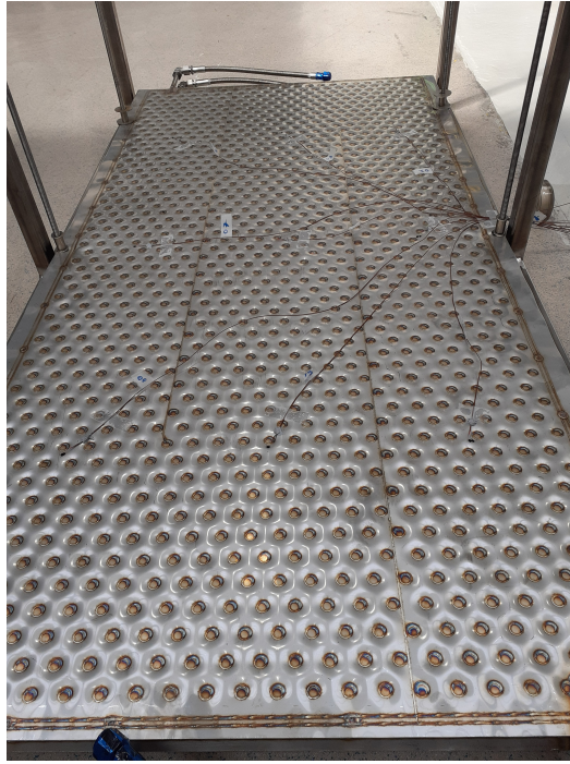
Figure 3.6: Location of thermocouples close to the PP surface on plate number 2, 5 and 9 in the stack (PP2 shown in the figure).
