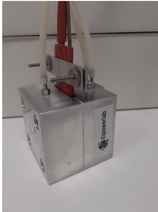
Figure 3.11: Experimental setup for measurement of thermal conductivity of liquid samples
