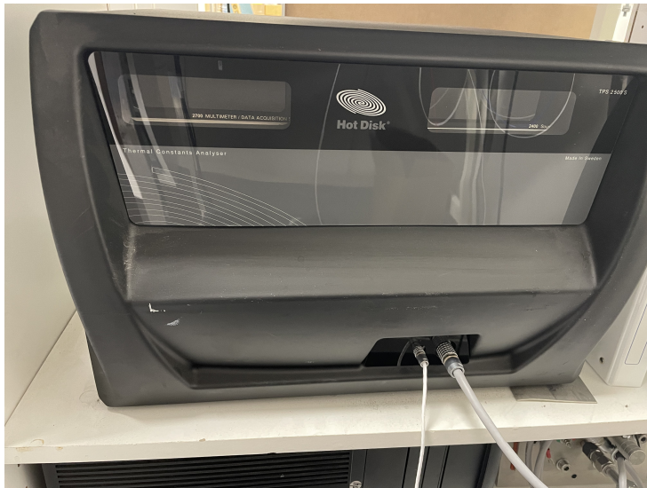
Figure 3.9: HotDisk TPS 2500S thermal constants analyser used for determining the thermal conductivity of PCM
