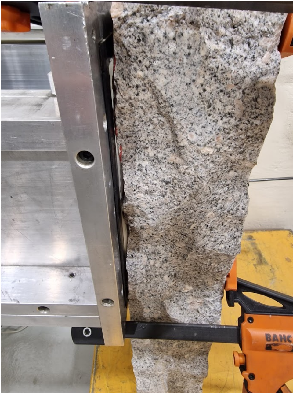
Figure 3.5: Sideview of "rough rock" to showcase unique sealing challenge due to the sample's shape.
