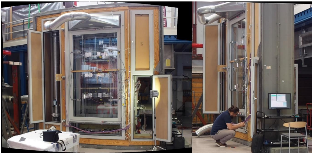
Fig. 1. – The DSF draws air from the lower opening and transfers it through the cavity to the upper opening. Further, the ventilation system attached to the upper vent takes the air first to the ultrasonic flow meter and then to the fan located in the vertical duct placed in the DSF’s side section. Finally, the air is expelled to the outside or inside as needed.
