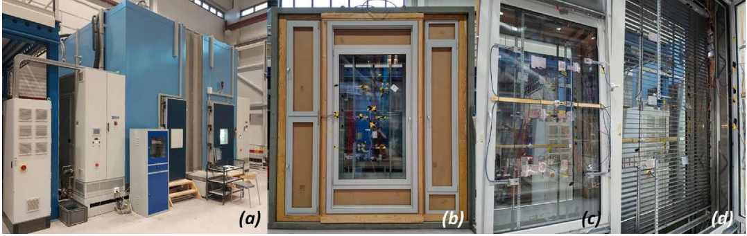
Fig. 2. Experimental set-up: (a) the climate simulator with the façade installed between the two chambers (and visible as the metal frame between the two blue cells); (b) frontal view of the DSF mock-up installed in the frame for insertion in the climate simulator facility; (c) and (d) sensors installation on the mock-up. (For interpretation of the references to color in this figure legend, the reader is referred to the web version of this article.).
