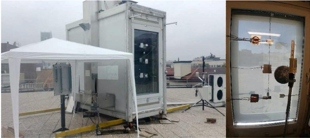
Fig. 1. An experimental set-up consisting of CO 2 -supply instrumentation, the DSF test sample, the automatic weather station (left) and the view from the inside of the cell (right).
