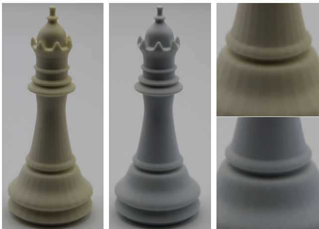
Fig. 16. A chess piece printed with flat (left) and PN-triangles (right).
