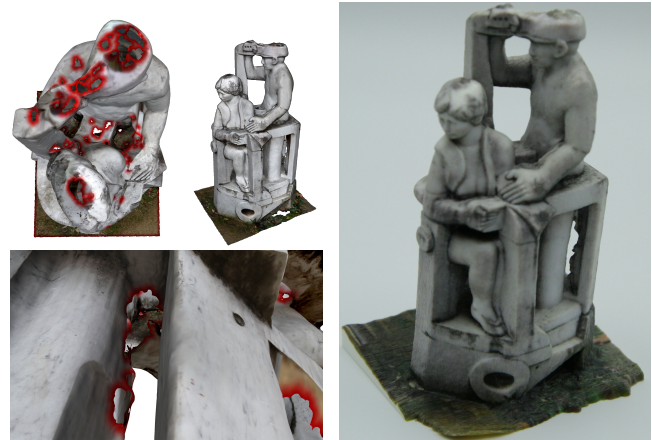
Fig. 9. This scan of a statue of Copernicus has many holes (boundaries highlighted in red), and is completely open on the bottom. The print on the right is neither missing structures nor introducing extraneous structures.
