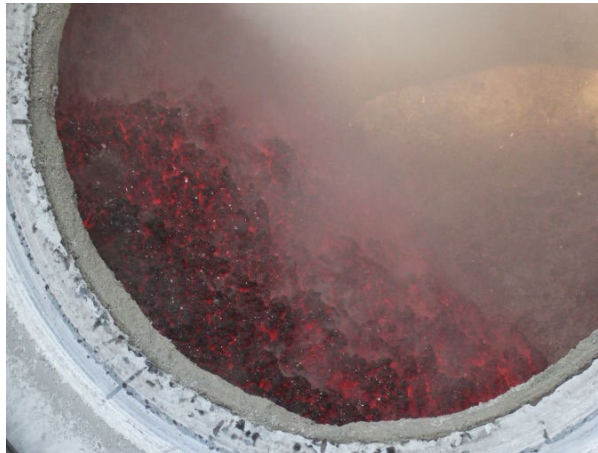
Fig. 4.5: Salt cake formed inside a rotary furnace. © International Mining 2022[100].
