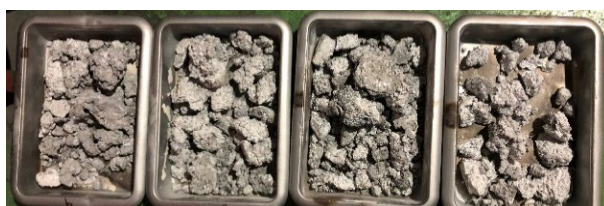
Fig. 5.2: Collected dross samples left to cool in the ambient air of the casthouse from Location 1 to Location 4.
