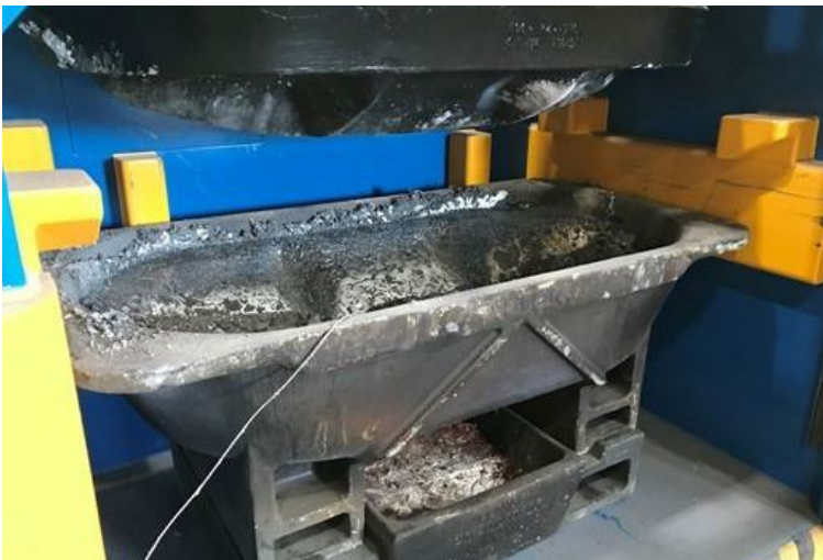
Fig. 4.11: Dross press with the metallic Al collected under the dross bin after the white dross has been pressed. © ALTEK[113].
