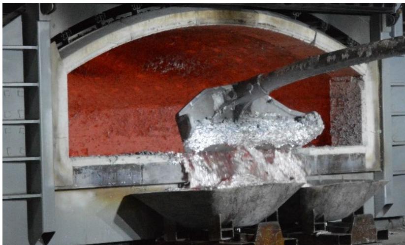
Fig. 1.2: Image of the skimming of an Al melt, where dross bins are placed in front of the furnace gate to collect the oxides and non-metallic compounds (NMCs) floating on top of the melt before casting. Metallic Al is entrained, generating Al-rich white dross. © 2021, Alcoa Mosjøen, Norway.
