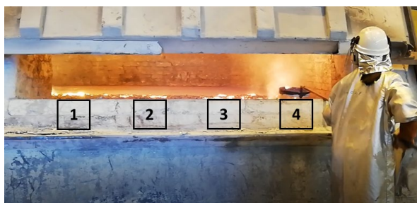
Fig. 5.1: Collection of dross samples from Location 1 (closest to the injection point of the primary produced Al) to Location 4 (furthest away) in the holding furnace using the 2-meter-long dross sampling tool. © 2019, Hydro Karmøy, Norway.
