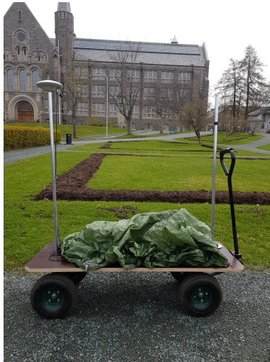
Figure 4.1: GNSS antennas, sensor suite and laptop with rain cover on trolley at test site.
