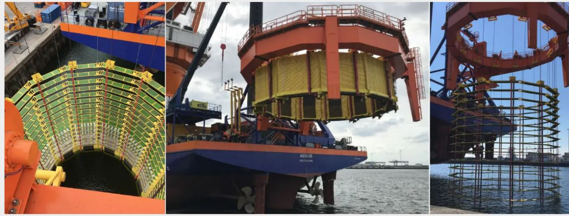
Figure 2.17: Noise Abatement System from AdBm Technology
