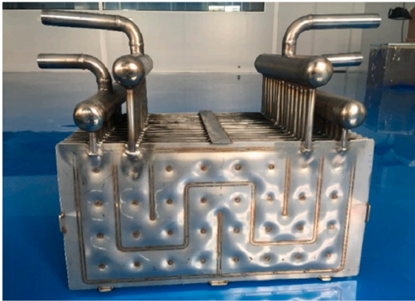
Fig. 14. Photographic view of the heat exchanger investigated by Lin et al. [59] (reprinted from Applied Thermal Engineering, 178, W. Lin, W. Zhang, Z. Ling, X. Fang, Z. Zhang, Experimental study of the thermal performance of a novel plate type heat exchanger with phase change material, 115630, Copyright (2020), with permission from Elsevier).
