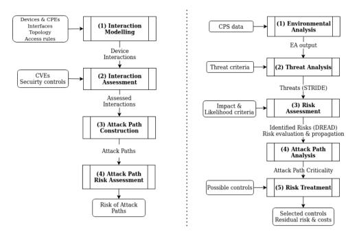
Figure 1. An overview of the underlying CPS RA methodologies of Stellios et al. [11] (left) and Kavallieratos et al. [13] (right).
