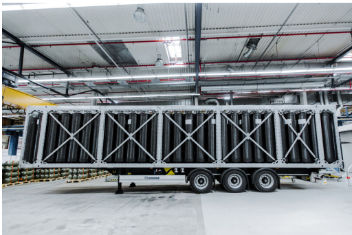
(a) Tube road semi-trailer by “Hexagon Purus” Source: hexagonpurus.com
