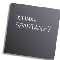
Figure 2: Xilinx Spartan-7 FPGA, illustration taken from [21]
