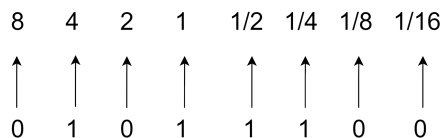
Figure 10: An example fixed point number 0100.1100 2 equalling 4.75 10
