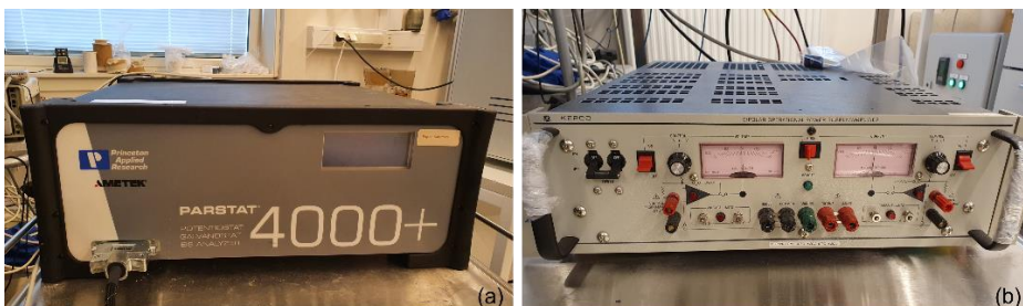
Figure 3.20. (a) PARSTAT 4000+ potentiostat and (b) KEPCO current booster.
