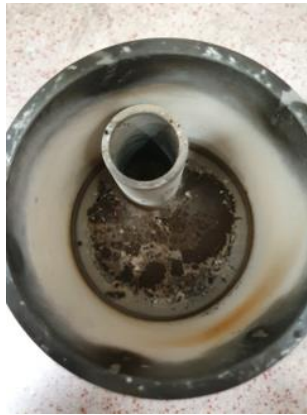
Figure 5.16. Picture of the surface of the frozen bath in the silicon nitride crucible at room temperature after the experiment with the rod anode and inverted horizontal anode.
