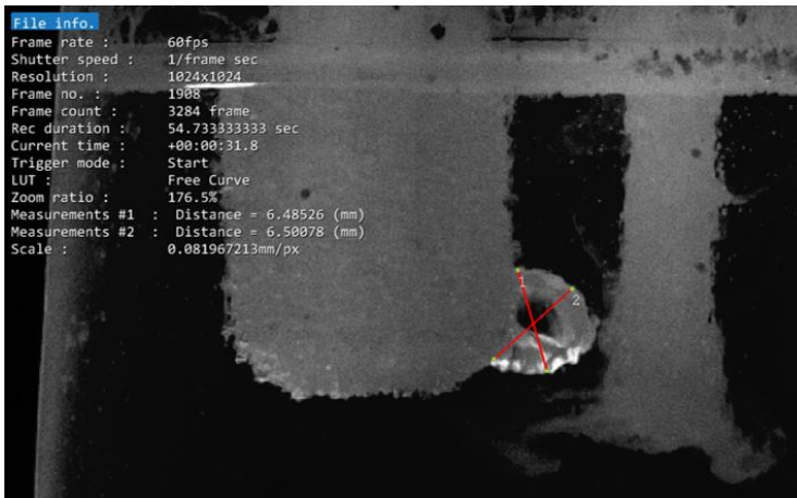
Figure 6.20. An example of measurement of the bubble diameter during electrolysis using the horizontal anode at current density 0.7\text{ A cm}^{-2} . The average value was used.
