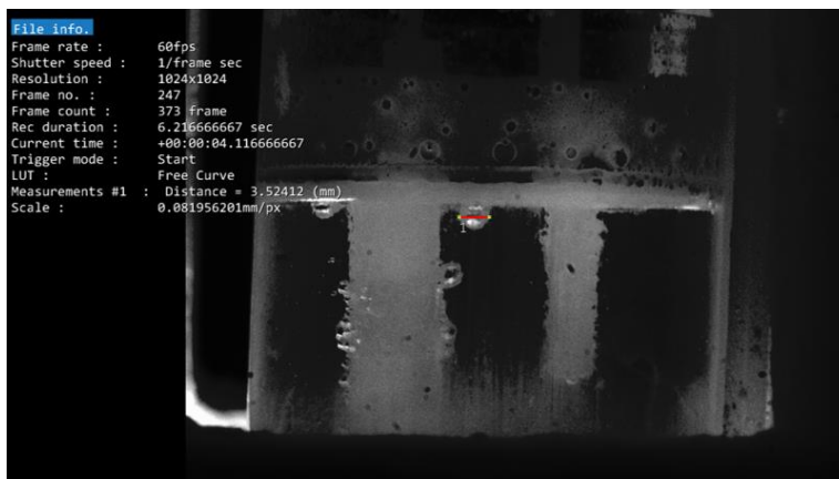
Figure 6.21. An example of measurement of the bubble diameter during electrolysis using the vertical anode at current density 0.25 \text{ A cm}^{-2} .
