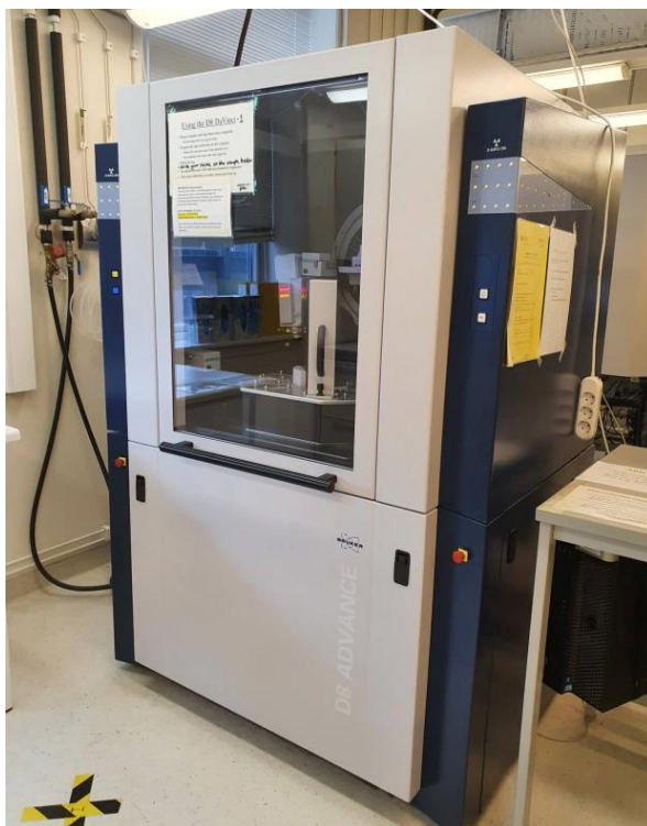
Figure 3.24. Bruker D8 A25 DaVinci X-ray Diffractometer with \text{CuK}\alpha radiation.
