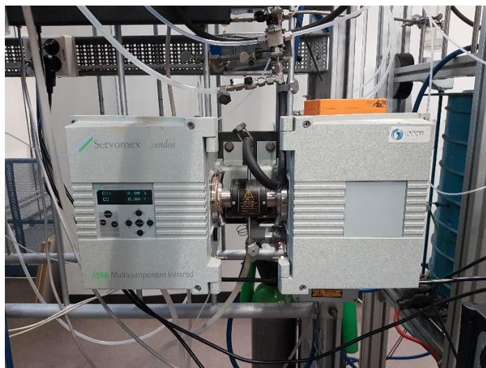
Figure 3.21. Servomex Xendos 2550-gas analyzer.
