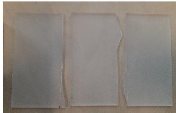
Figure 5.1 inaccuracy of cutting of samples
