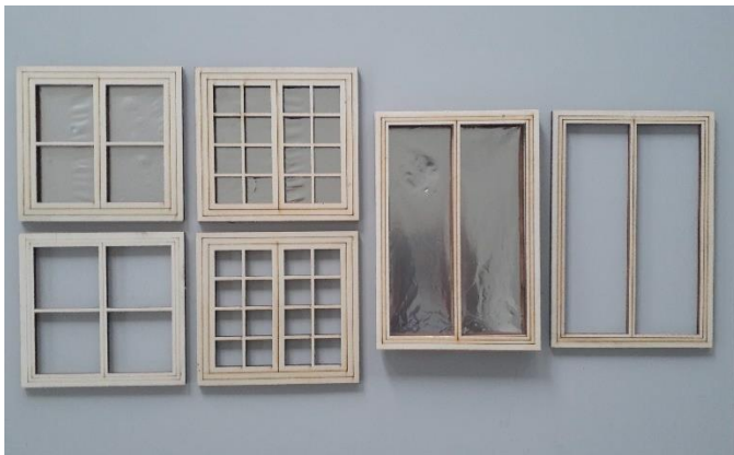
Figure 3.12 Doors and windows cut out of plywood and lined with aluminum foil
