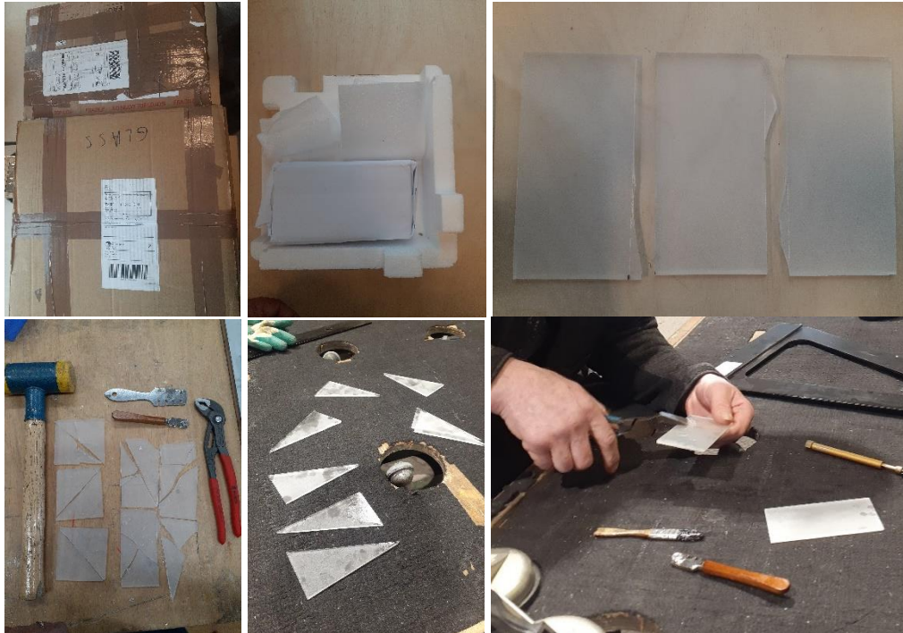
Figure 3.14 cutting of glass samples into required shape and size.
