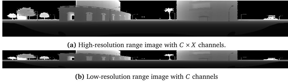
Figure 3.2: Example of how the high-resolution range image (a) and low-resolution image (b) are generated. Initially a lidar with C \times X channels is simulated to generate the high-resolution range image. Then every X -th row is extracted to generate the low-resolution image. In this illustration we have that C = 64 and X = 2 .
