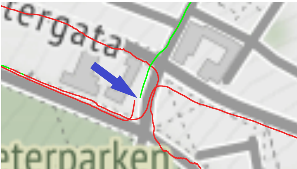
Figure 4.3: An example from the Trondheim Urban dataset where the GNSS data "jumps" when the GNSS receiver converts from standard GNSS positioning (red) to RTK positioning (green). Map tiles by © Stamen Design, under CC BY 3.0. Data by © OpenStreetMap, under ODbL.
