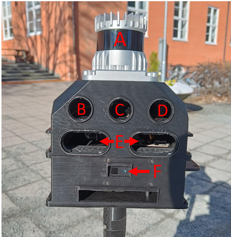
Figure 3.15: Front side of the Mjolnir sensor rig, where we see: (A) an OS0-128 lidar. (B-D) Slots for three mono cameras. (E) Slot for a ZED 2 stereo camera, which was installed later. (F) A CamBoard pico flexx depth camera.
