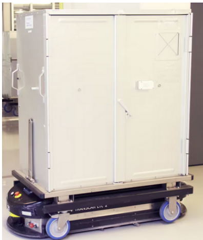
Figure 4.1: Automated Guided Vehicle transporting a cart at St. Olavs Hospital
