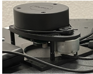
Figure 2.2: RPLIDAR A1 mounted on top of Alfred
