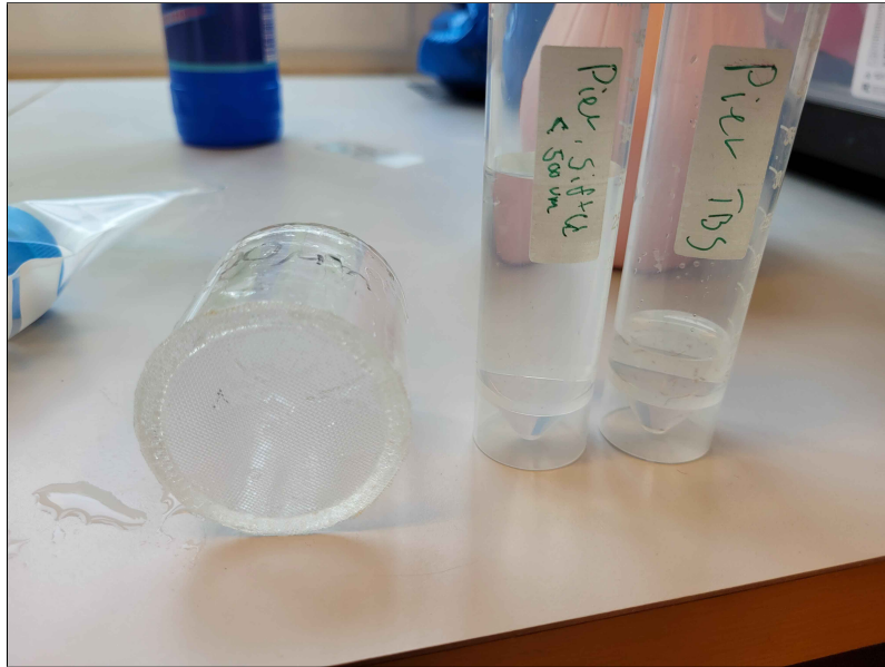
Figure 28: A sieve with a mesh size of 500\mu\text{m} . All samples were filtered through this sieve such that the particle size would be in the range 50\mu\text{m} - 500\mu\text{m} .
