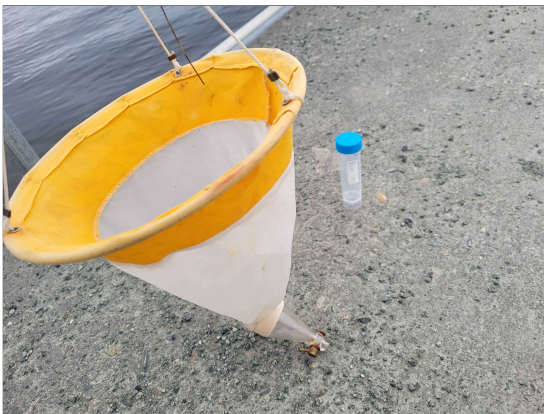
(a) Plankton net and sample container.
