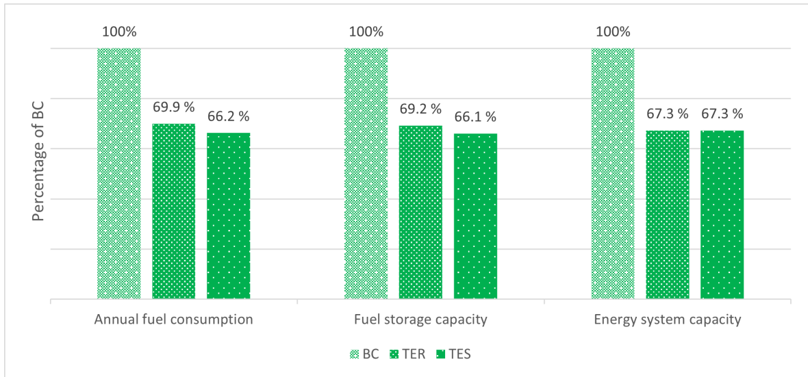
Figure 20: The effect of including TER and TES on annual fuel consumption, fuel storage capacity, and energy system capacity.
