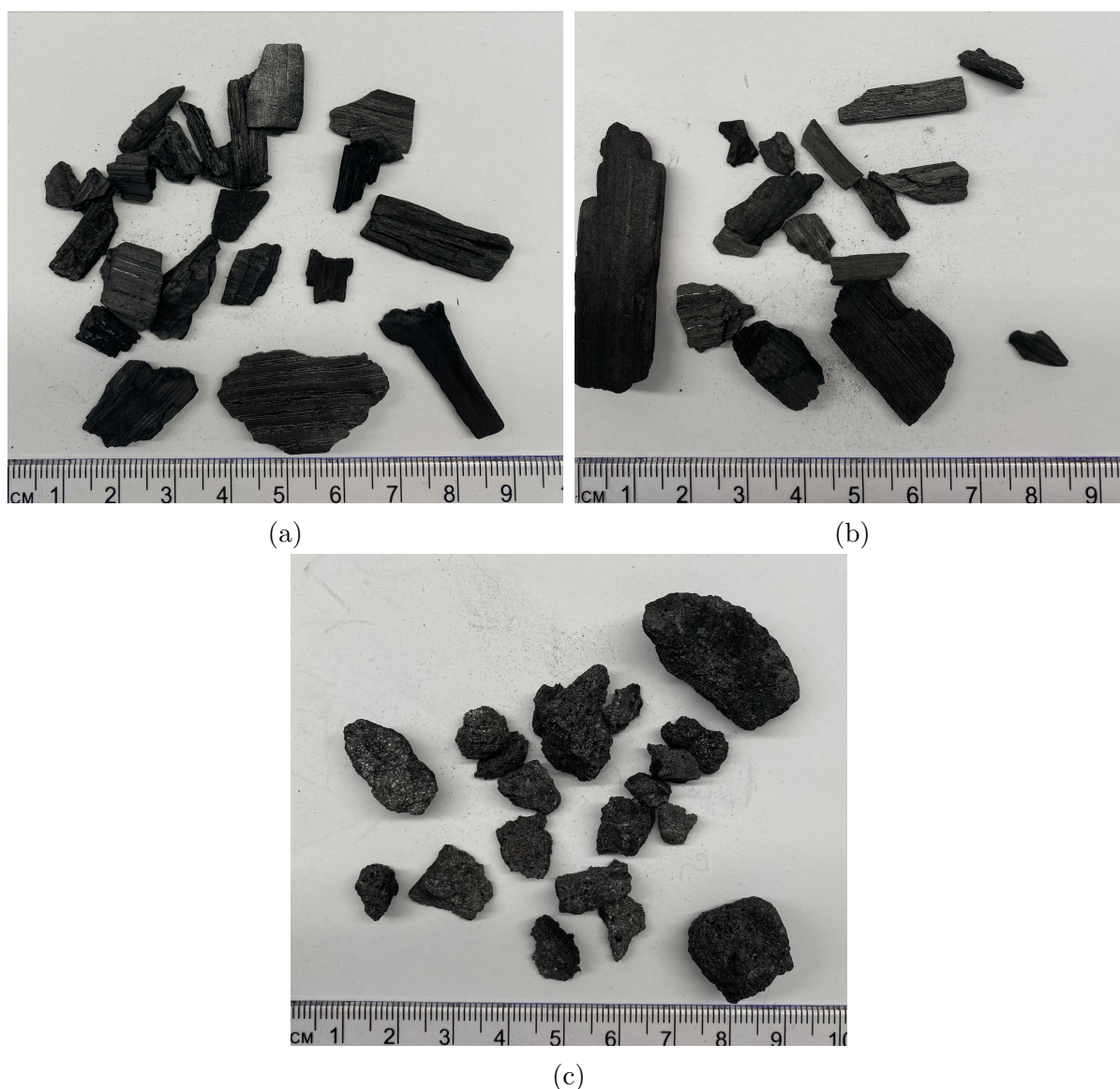
Figure 3.1: The raw materials showed with size distribution of 5-16 mm. Figure (a) is CharcoalRM, Figure (b) is CharcoalHT and Figure (c) is Coke.
