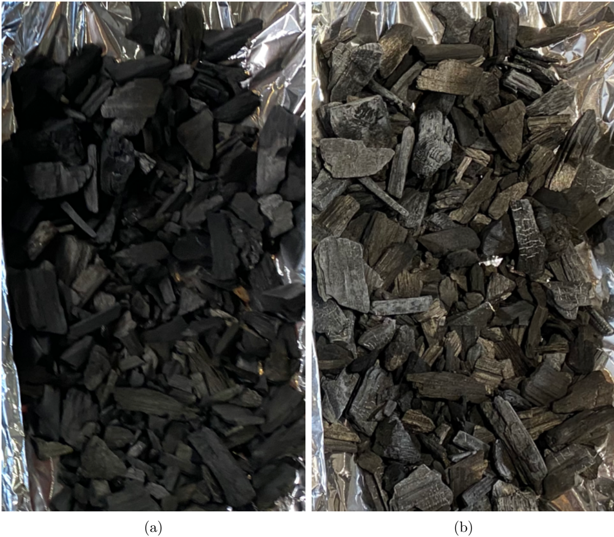
Figure 3.7: Photo of the charcoal right after the sample is unloaded and divided by layers (a) after the K-impregnation, and the charcoal after the unloading where the K-impregnated sample have been able to oxidize in air for 2h (b).
