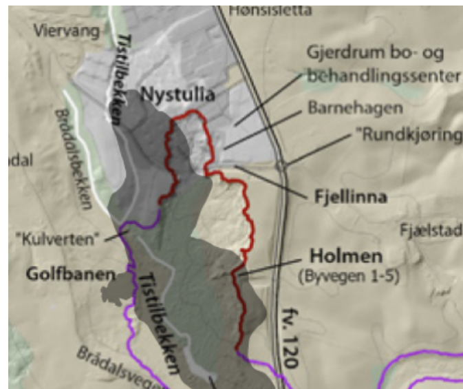
Figure 6.21: Extent of slide in simulation 3. Background map with outline of detachment area (red) and run-out area (purple) from Ryan et al. (2021).
