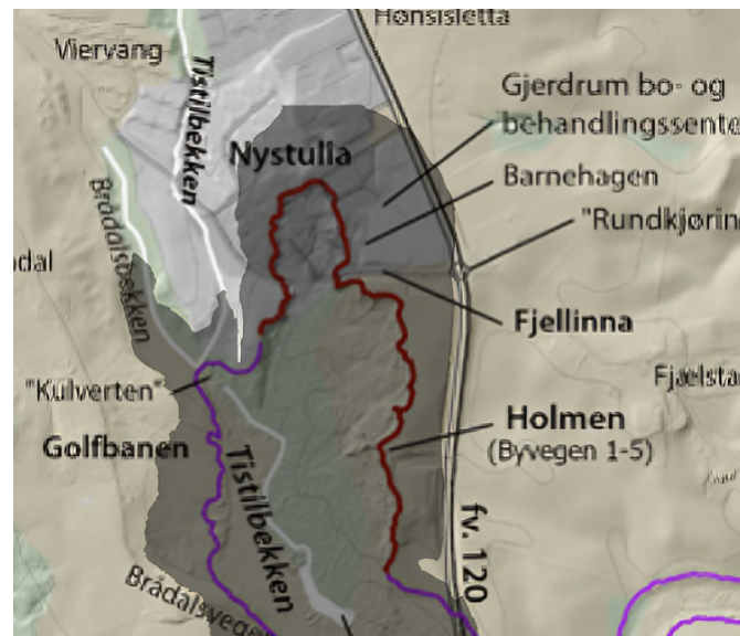
Figure 6.14: Extent of slide in simulation. Background map with outline of detachment area (red) and run-out area (purple) from Ryan et al. (2021).
