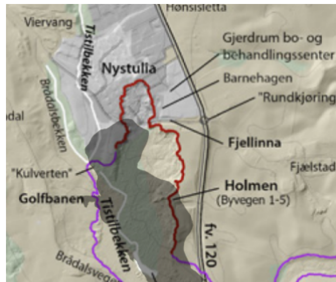
Figure 6.17: Extent of slide in simulation 2. Background map with outline of detachment area (red) and run-out area (purple) from Ryan et al. (2021).
