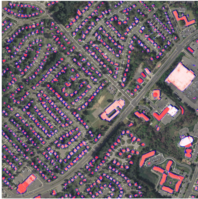
Figure 2.2: Building extraction using deep learning semantic segmentation. [30]
