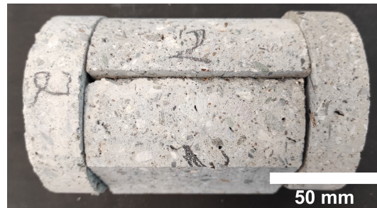
Figure 7: Parts of core used for PF and IMA. The outer discs were used for PF and the half cylinders for IMA.
