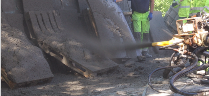
Figure 6: A panel which was sprayed 67/23 degrees to the panel surface. Photo: Nicholas Henry Trussell.
