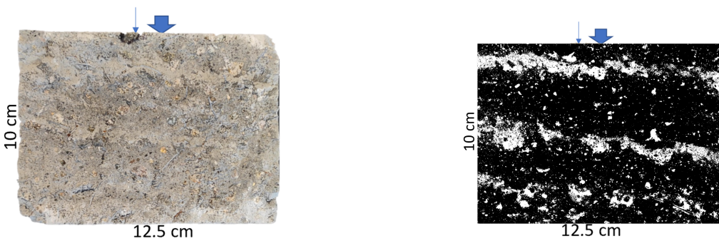
(a) Water penetration front of the 10%P5-cube.
