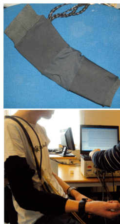
Figure 3.7: Textile electrode sleeve for recording of HD-sEMG signals. From [16].
