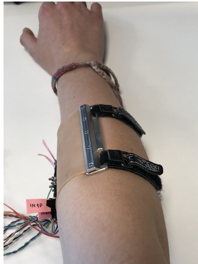
Figure 5.1: Adjustable attachment mechanism of the sleeve consisting of aluminium braces and velcro straps.
