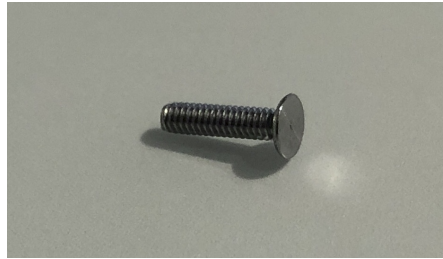
Figure 5.3: Final shape of the electrodes used for the prototype.
