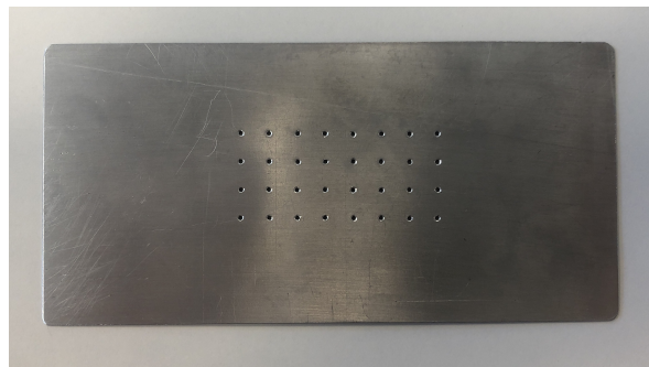
Figure 5.5: The grid template used to make holes in the sleeve. The grid is 4x8 and has a distance between holes of 5.5mm.
