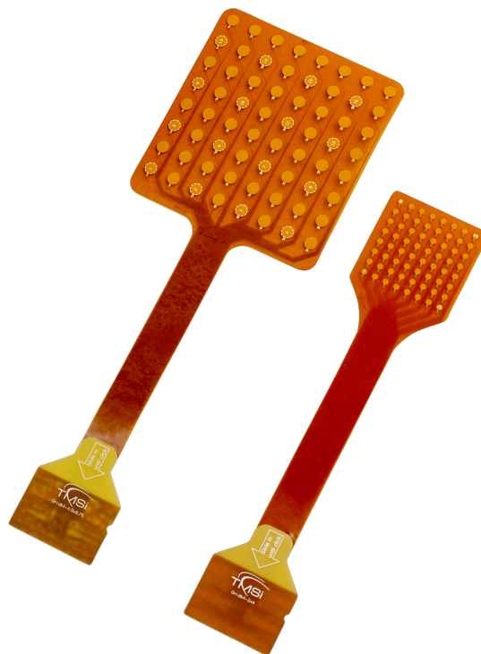
Figure A.5: TMSi HD-EMG electrode grids. From [50].
