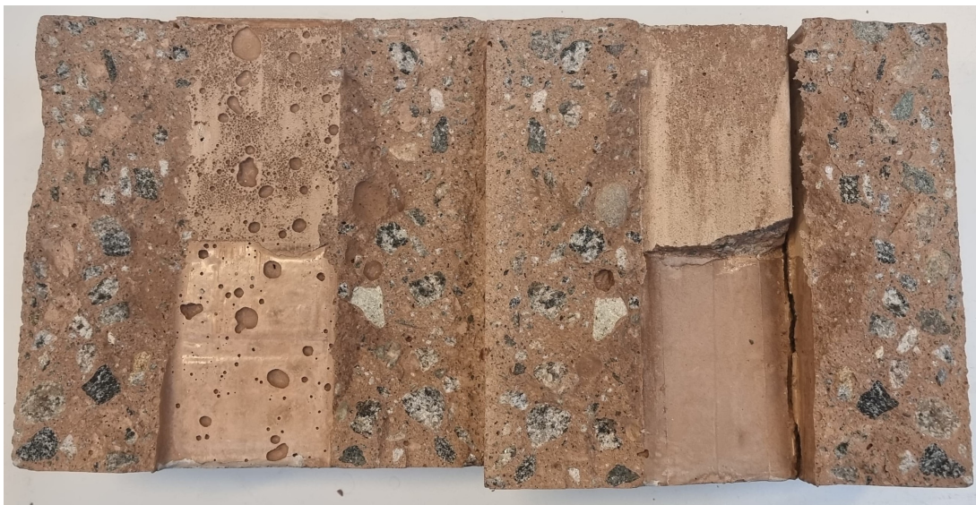
(b) Cement imprint for L-shape reinforcement
