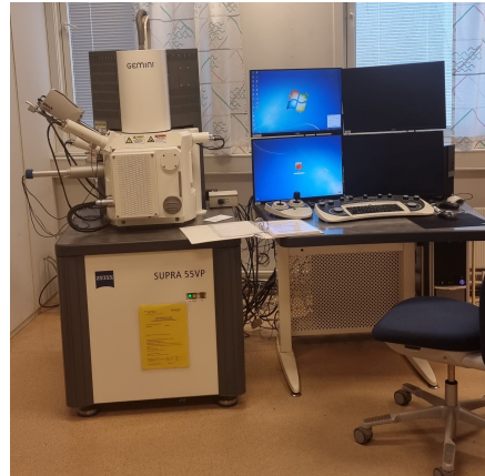
(f) Image of the SEM-EDS machine Zeiss-Ultra 55
