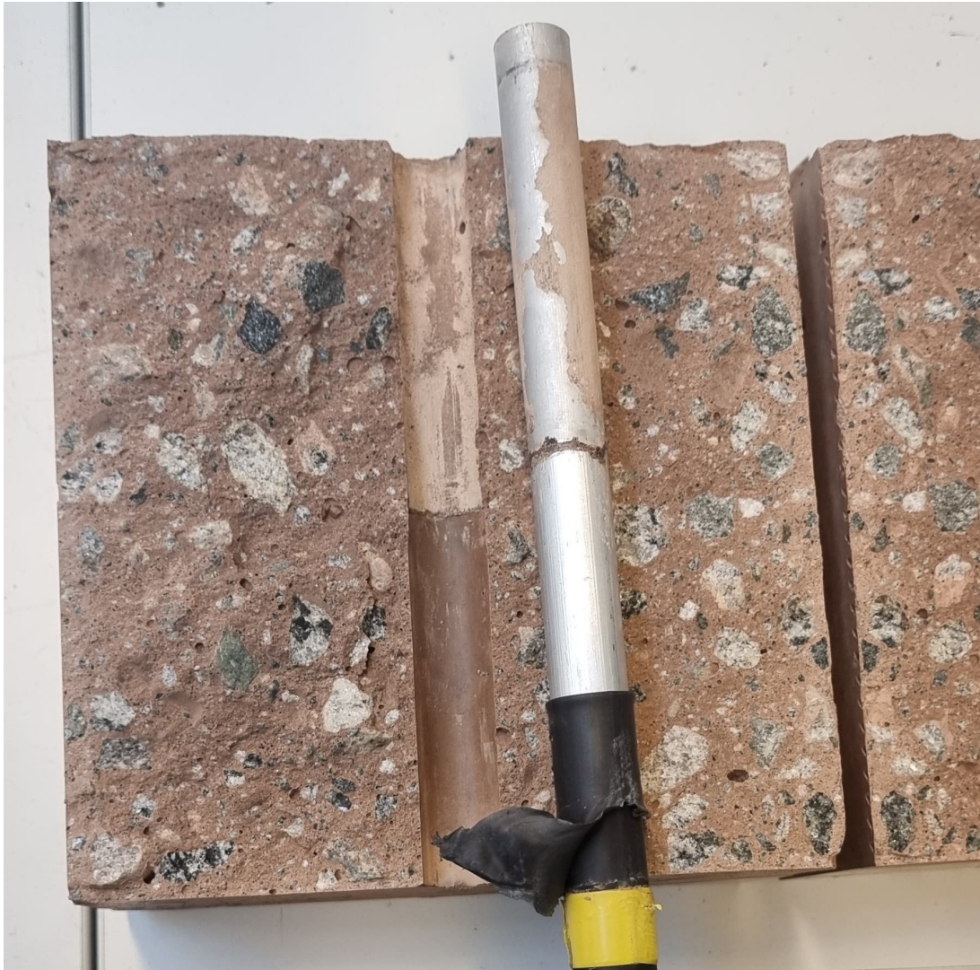
(a) 6082 bar after pull-out and corresponding cement imprint
