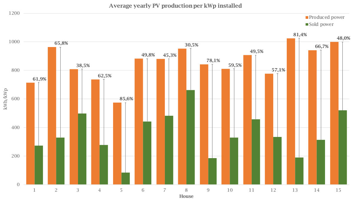
Figure 5.6: Average yearly PV production for each residence, the amount they sold, and percentage of self-consumption, based on data from 2021.
