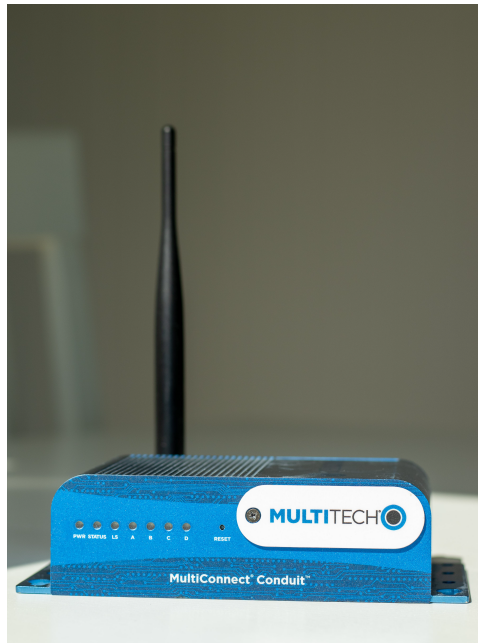
Figure 4.6: MultiTech Conduit LoRa Gateway used as basestation. Photo: E. Jølsgard/NTNU
