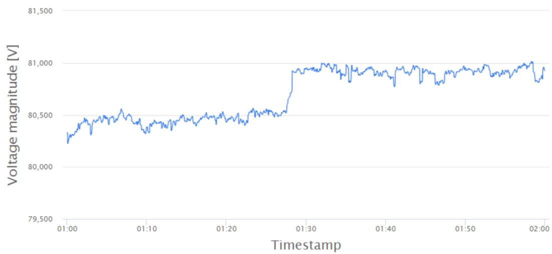
Figure 33: Median filtered phase voltage, M = 150 .
