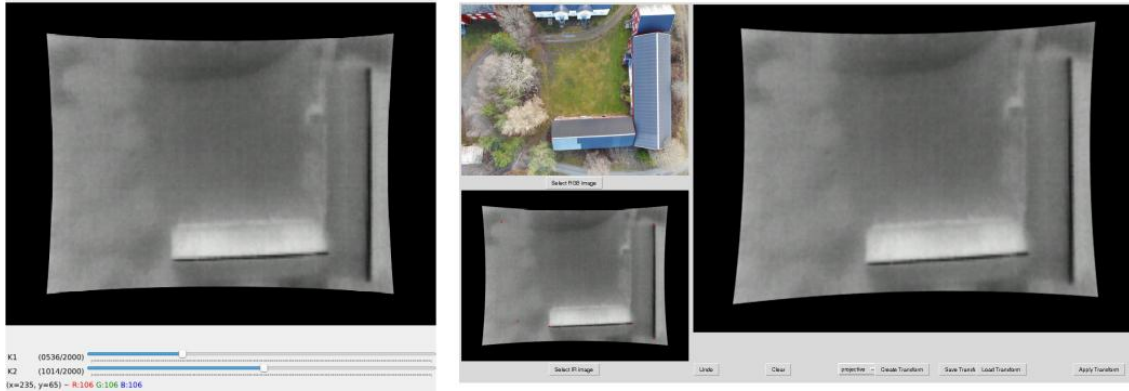
Figure 4.11: Sliders to used to control the K variables used for distortion correction. A GUI program using a slider to correct the distortion and the estimate_transform method from the Skimage toolkit to estimate the transformation between the two images.
