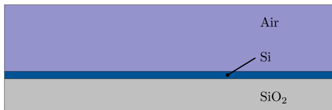
Figure 4.1: The effective mode index method COMSOL model. The model consists of a 10\ \mu\text{m} long structure, with a 1\ \mu\text{m} bottom \text{SiO}_2 layer, in turn with a 220\ \text{nm} thick layer of Si on top, representing the waveguide structure. The top air layer has a thickness of 2\ \mu\text{m} .
