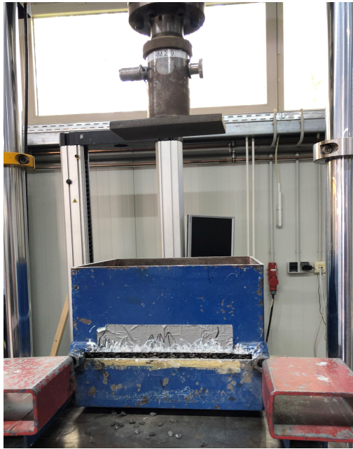
(a) System with loading plate, test container and aggregate in the lower part
