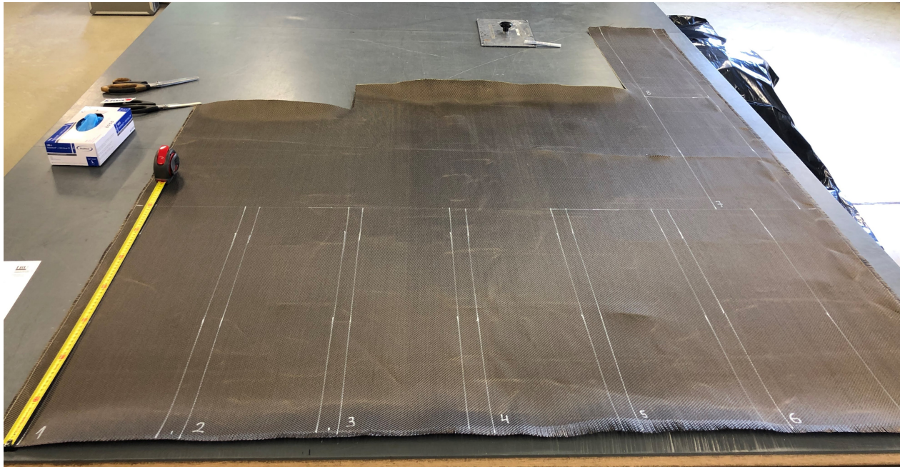
Figure 5.3: Preparation of test specimens on EB geotextile
