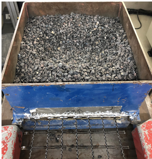
(c) RT geogrid after testing
