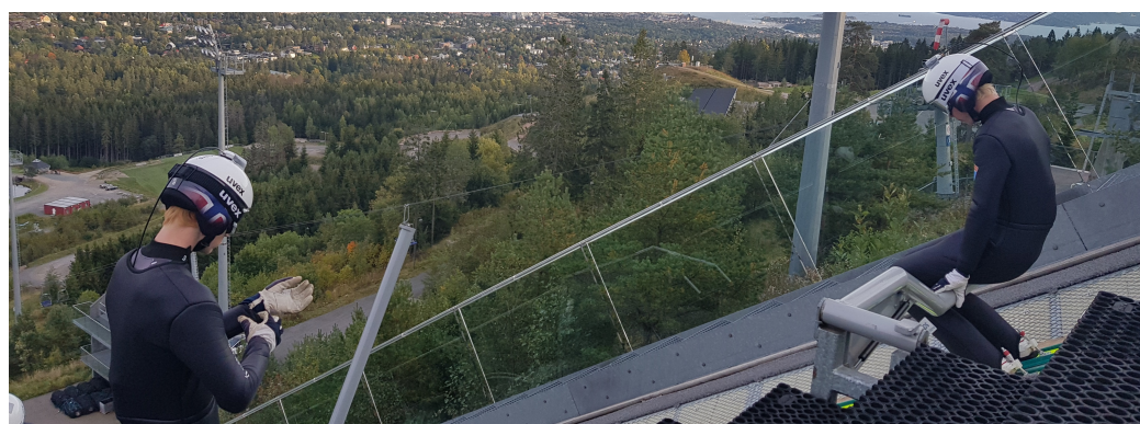
Figure 2. Ski jumpers with the dGNSS antenna mounted on their helmets and the receivers in backpacks that were carried under the ski jumping suit. Picture from [35].
