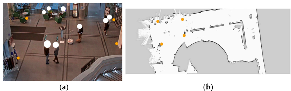
Figure 4. CCTV camera calibration: Yellow markers represent (a) pixel coordinates in angled view; (b) Cartesian coordinates in top view.
