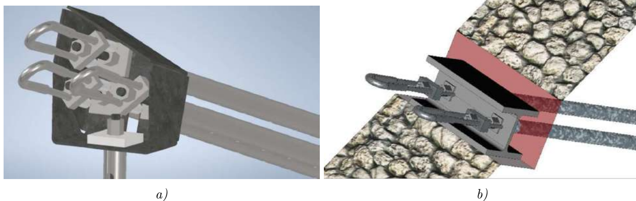
Figure 8.6: Drawing of what a) an anchoring "house" for the support ropes and b) an H-beam anchoring node for the retaining ropes could look like. From Jónsson [102, pp. 24, 25].
