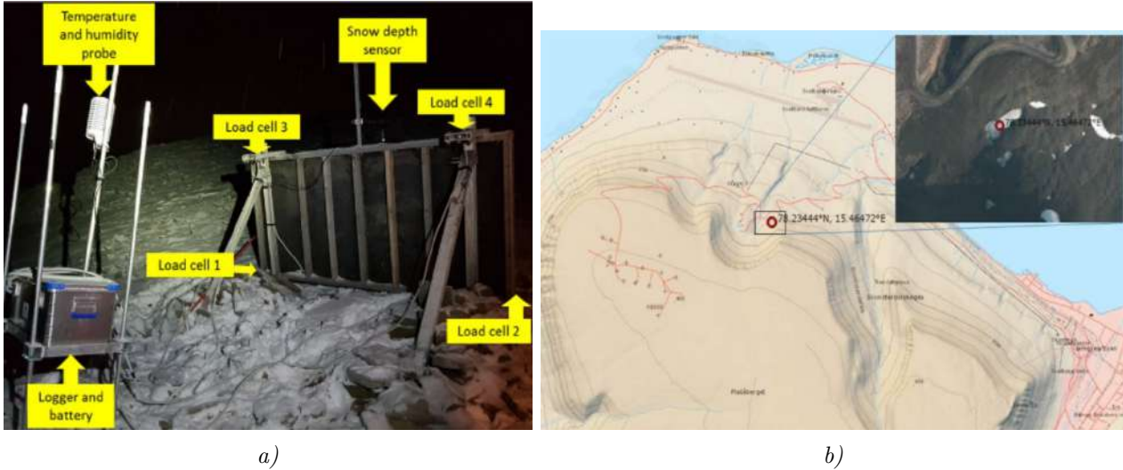
Figure 7.3: An overview of the original experimental setup of the Snow Load Testing System (a) and the location of the system between Longyearbyen airport and Platåberget (b). The setup currently being used has been slightly adapted compared from (a). Source: Arctic Technology Departmen, UNIS [96].
