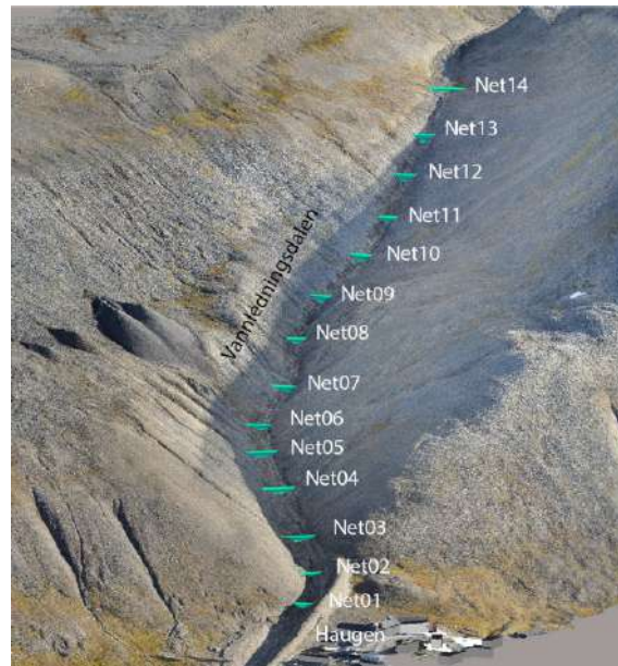
Figure 8.7: Planned barrier placement in Vannledningsdalen. Source: Jónsson [102].
