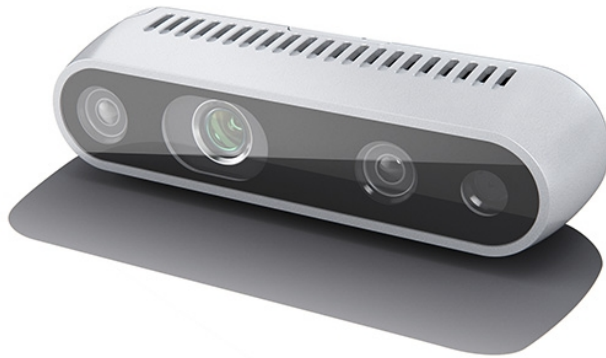
Figure 3.3: The stereoscopic depth camera
