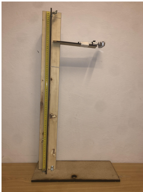
Figure 3.2: The plywood camera stand for hand gesture detection.
