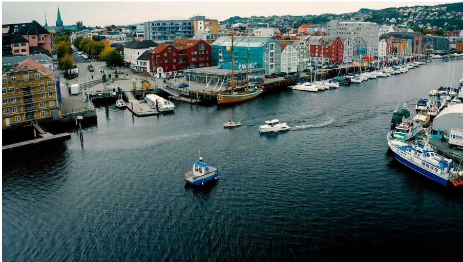
Figure 1: The milliAmpere (blue in the middle), a prototype of an autonomous electric passenger ferry, during testing of multi-target tracking performance in a canal area in Trondheim in November 2020. Two other vessels (upper right relative to milliAmpere) are used as target ships. Courtesy of Mikael Sætereid.
