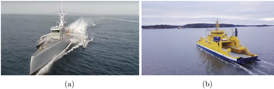
Figure 1.1: Some examples of early maritime autonomous vessels. (a) The DARPA prototype vessel Sea Hunter , developed for unmanned and autonomous anti-submarine operations [7]. (b) The world’s first autonomous car ferry Falco . Photo is from [8].
