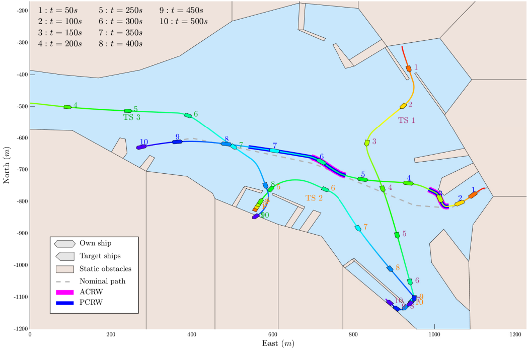
Figure 18: Simulation 3: Transit between two docking locations, with a give-way crossing, stand-on crossing and a head-on/give-way encounter.
