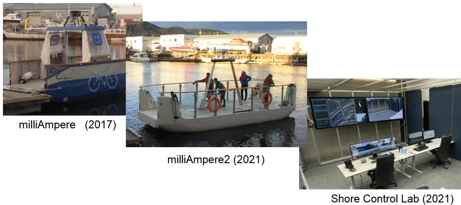
Figure 1.3: The unique equipment that the Autoferry project has contributed to establish and has access to. The milliAmpere is a prototype electric autonomous passenger ferry. It is named after the world's first all electric car ferry Ampere [20]. The milliAmpere2 is a full-scale electric autonomous passenger ferry that is planned for trial operation in Trondheim in 2022. The Shore Control Lab is an advanced infrastructure for research and development in remote monitoring and control of autonomous maritime systems, and human-machine interaction.
