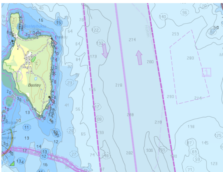
Figure 6.2: Screenshot of Traffic Separation Scheme displayed together with a ENC chart outside Horten, Norway [100].
