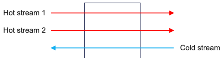
Figure 3.2: Multistream heat exchanger.
