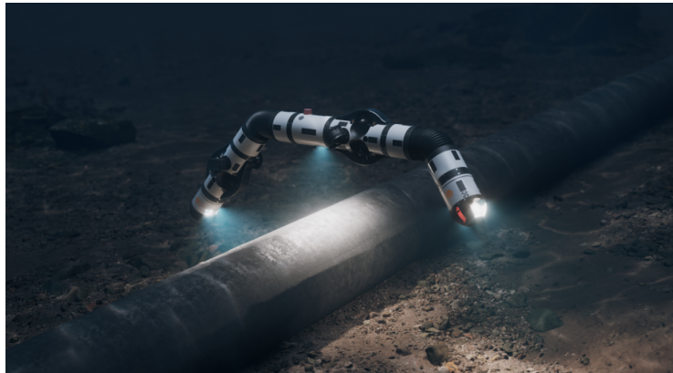
Figure 1.2: Eelume robot inspecting a subsea pipeline. (Eelume 2022).
