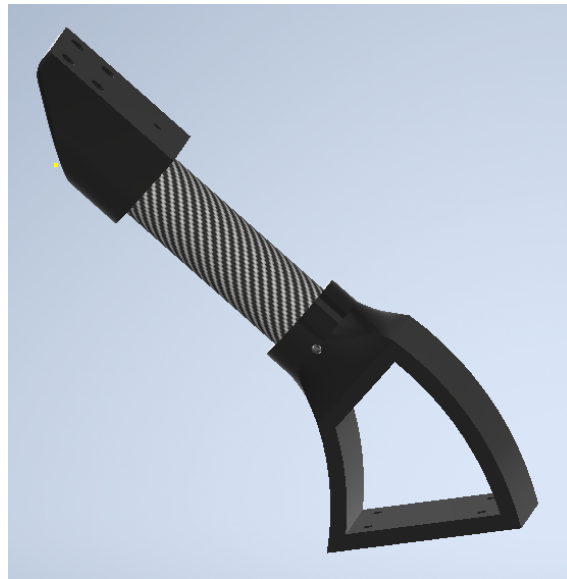
Figure 4.21: Assembled Changeable Sole Paw, with a carbon fiber pipe as the adjustable length part.
