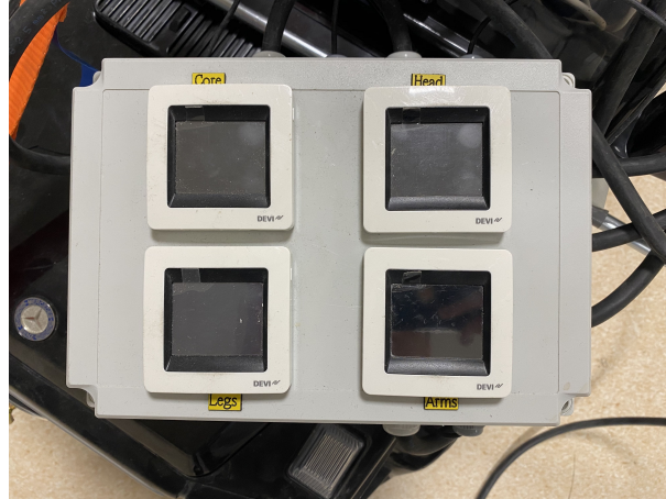
Figure 3.12: Equipment to heat up the exposed manikin to skin surface temperature.
