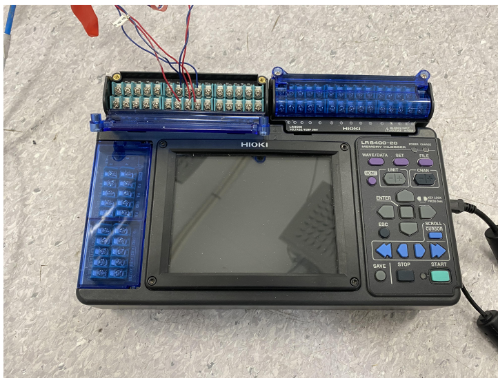
Figure 3.16: Memory HiLogger to monitor temperature.
