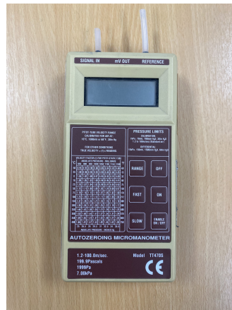
Figure 3.14: Autozeroing micromanometer model TT470S to measure the pressure difference in the supply air diffusers.
