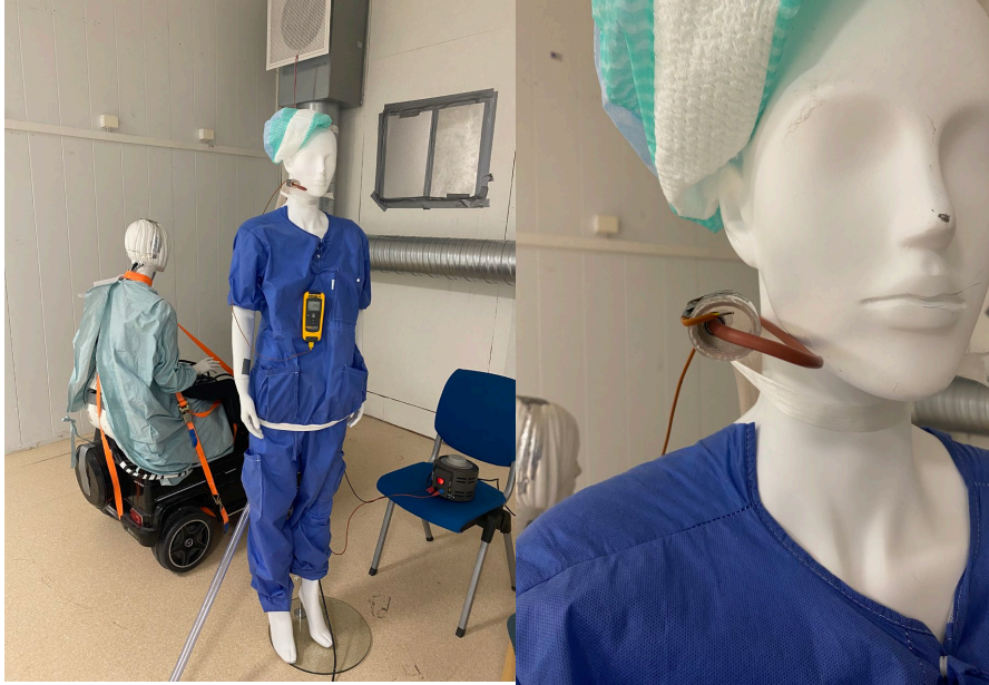
Figure 1: Manikin simulating an infected teacher. The tube close to the manikin's mouth will be put through the manikin's mouth (with a bored hole). Inside the tube there is a heating element to heat the exhaled air. Right-hand side picture shows this close-up.
