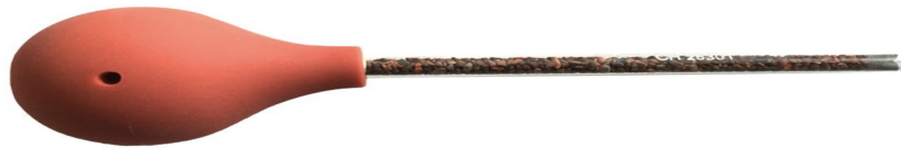
Figure D.1: Drager Air-Flow Tester kit for smoke visualization of exhaled jet.
