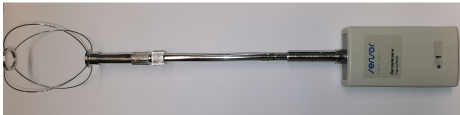
Figure 3.18: SensoAnemo 5100LSF to measure velocity of the exhaled jet from the infected manikin.
