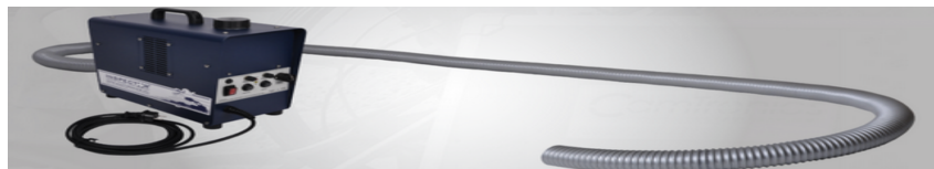
Figure D.2: Manual EasySmoker to visualize the airflow pattern in the laboratory.
