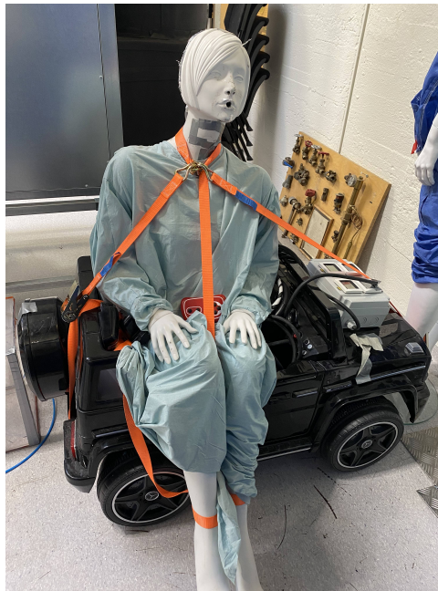
Figure 3.11: Manikin simulating a sitting exposed person.
