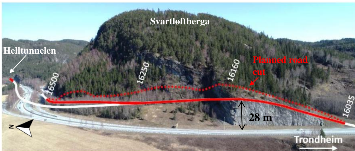
Figure 1.1: Overview map of the current road cut at Hommelvik, centre line for the new E6 highway (red line for planned road cut and white line for the rest), and the top of the planned road cut (red dotted line). It should be noted that the red to the left in the figure represents the tunnel portal at Helltunnelen. Modified after Multiconsult Norge AS (2019a).
