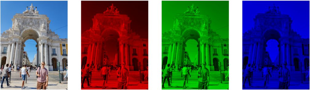
Figure 2.2.: a 3 \times 3000 \times 4000 RGB-image, where each channel corresponds to the amount of red, blue and green in each pixel. Every channel has values ranging from 0-255, depending on the intensity of the pixel. Photograph taken by me
