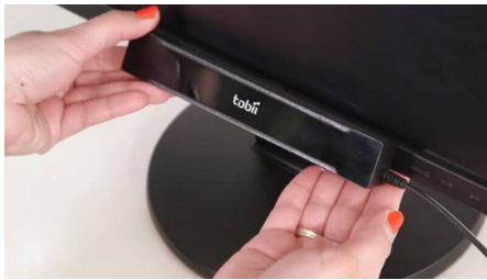
(a) Table-mounted eye tracker from Tobii connected to a desktop computer screen.
