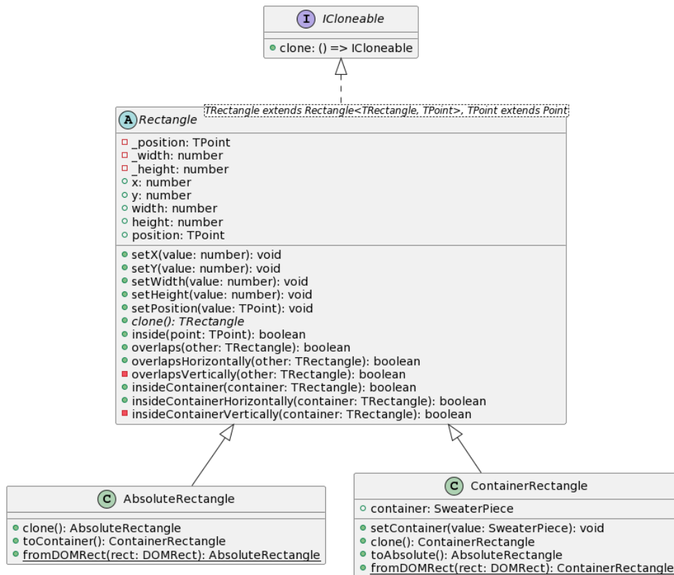
Figure A.1: Class diagram of types representing geometric rectangles (React Prototype 3).
