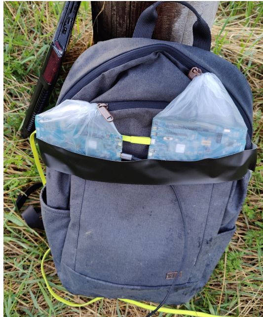
Figure 4.8: Backpack with two nRF52833 Development Kits attached to the outside.
