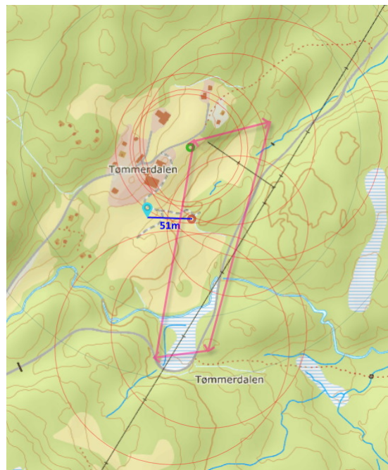
Figure 4.34: For 03.06, true location of Development Kit (Cyan marker) vs. estimated location (red circle) with RTT distance estimates and the flight path of flight 4 plotted in.
