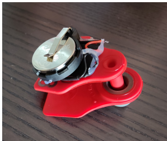
Figure 3.5: Second version of our prototype tag. It was additionally wrapped in a thin plastic bag for water protection, and taped to the ear tag.
