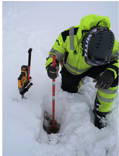
Figure 3.8: Installed measure pole for time-lapse camera at Hiorthamn. Picture taken by author.
