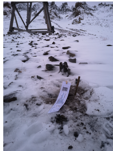
Figure 3.6: Installed i-button, from installation in February 2022. Picture taken by author.
