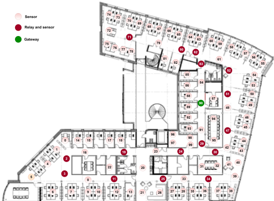
Fig. 5. The sensors, relays, and the gateway in the test-bed. Each circle with a number inside represents the approximate placement of each node and the number represents the node ID.
