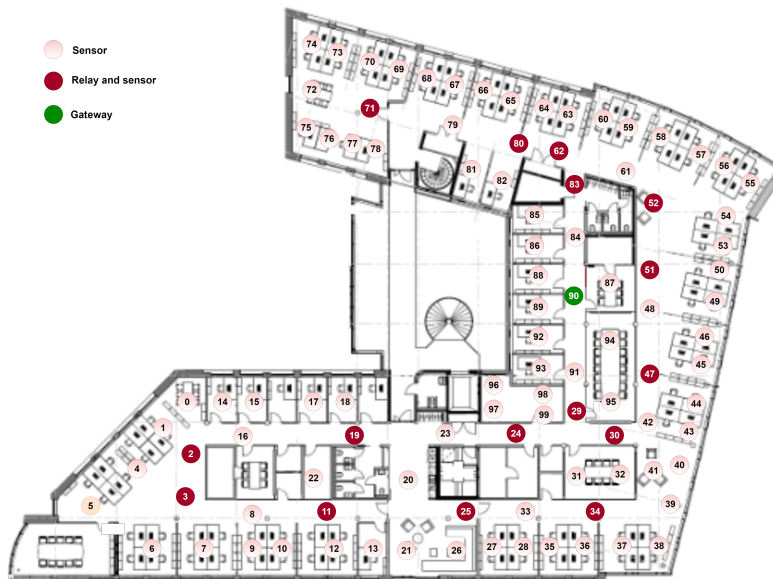
Figure 6.4: The sensors, relays, and the gateway in the test-bed. Each circle with a number inside represents the approximate placement of each node and the number represents the node ID.
