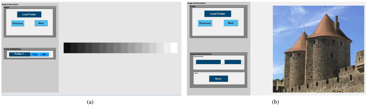
Figure 3. The test was conducted by running the GUI file in MATLAB. (a) Checking that the observer is able to clearly distinguish between the 16 brightness levels in the image. (b) Observer enhances the image using the sliding bar.
