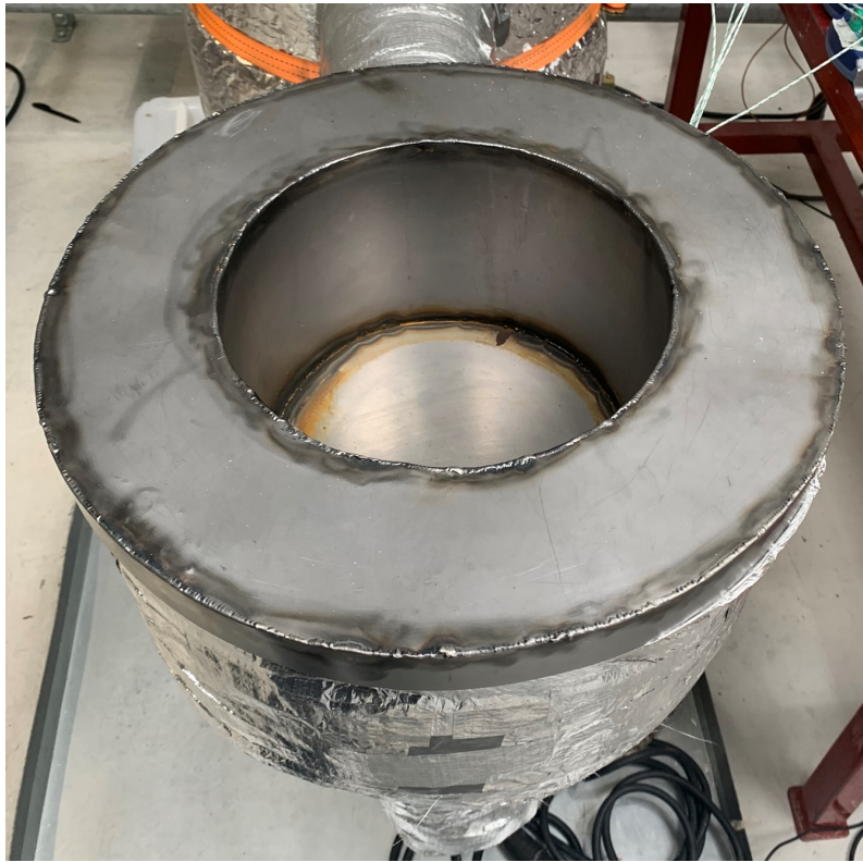
Figure 5.7: New cooker top without spacers and external insulation
