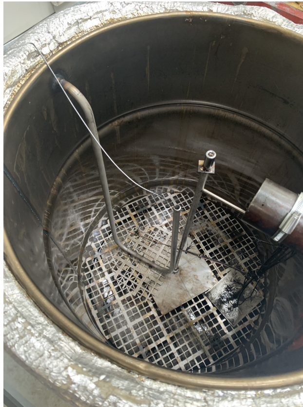
Figure 5.5: Guide tube and top of pump in empty modified SHTES
