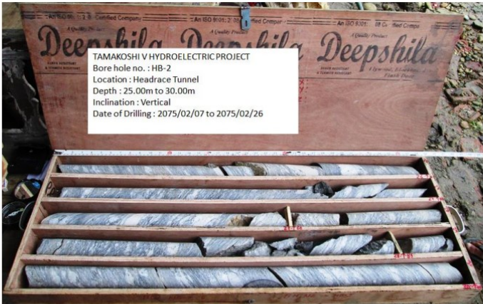
BOREHOLE NO. HB – 2', BOX NO. 6 OF 13, FROM 25.0 TO 30.0m
