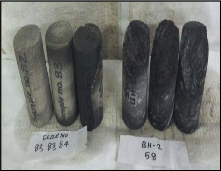
Figure 12-19: a View of Crushed Rock Core Samples after Triaxial Test
