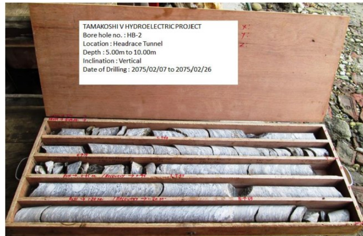
BOREHOLE NO. HB – 2', BOX NO. 2 OF 13, FROM 5.0 TO 10.0m
