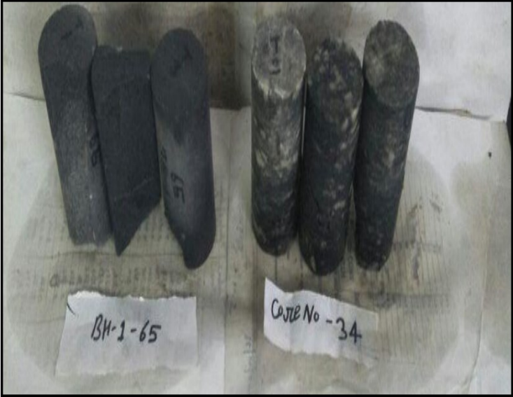
Figure 12-18: View of Crushed Rock Core Samples after Triaxial Test
