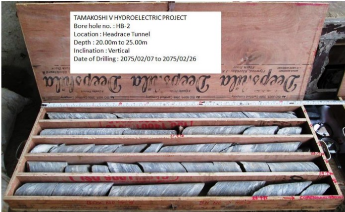
BOREHOLE NO. HB – 2', BOX NO. 5 OF 13, FROM 20.0 TO 25.0m
