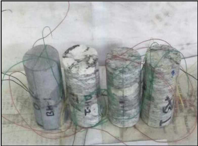
Figure 12-10: View Rock Core Sample before Modulus of Elasticity & Poisson's Ratio
