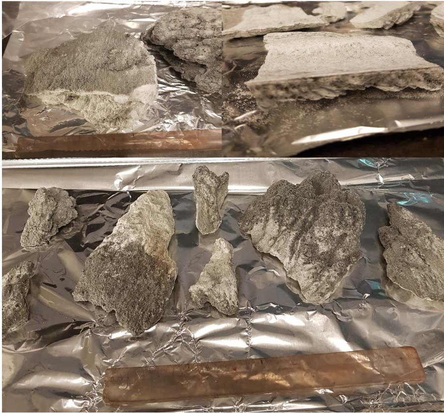
Figure 11: Raw sample from Furnace 2 all three samples are from the hot pipe where only the top right sample is closest to the furnace.
