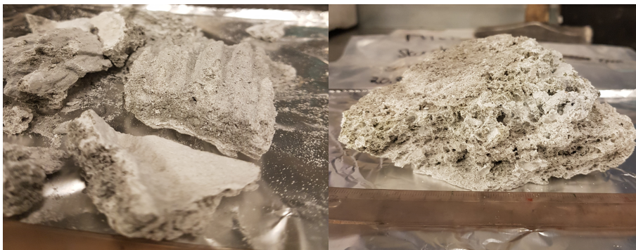
Figure 12: Raw sample from Furnace 2 both samples are from the colder pipe where the right sample is closest to the furnace.
